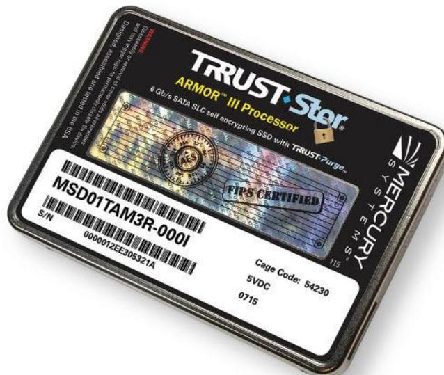
The one-terabyte TRUST-StorR SATA SLC self-encrypting solid-state drive (SSD) from Mercury Systems offers data protection and data management, protection from silent data corruption, and operational stability during power interruptions.
